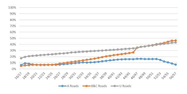
*Figure 4.8.2.2 Option IF2 change in percentage of roads in poor condition with additional £1.0M per annum from 2018/19 onwards*
