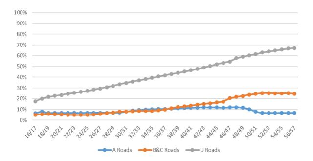
*Figure 4.7.2 Option BAU2 change in condition with current budgets with budget set aside to treat 5% of the backlog on Unclassified Roads*
