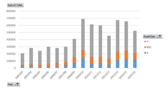
Figure 4.5.1 Expenditure on reactive repairs to carriageway surfaces by road class
